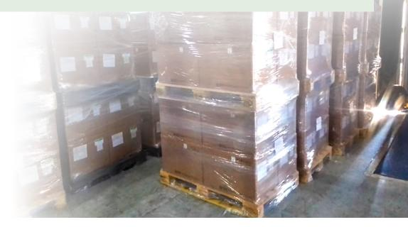
Double stacking, which was identified through PFSCM's Load Optimization, will save about 10% on the freight cost of one particular kind of RDT; the initiative also eliminates extra work further down the supply chain.
